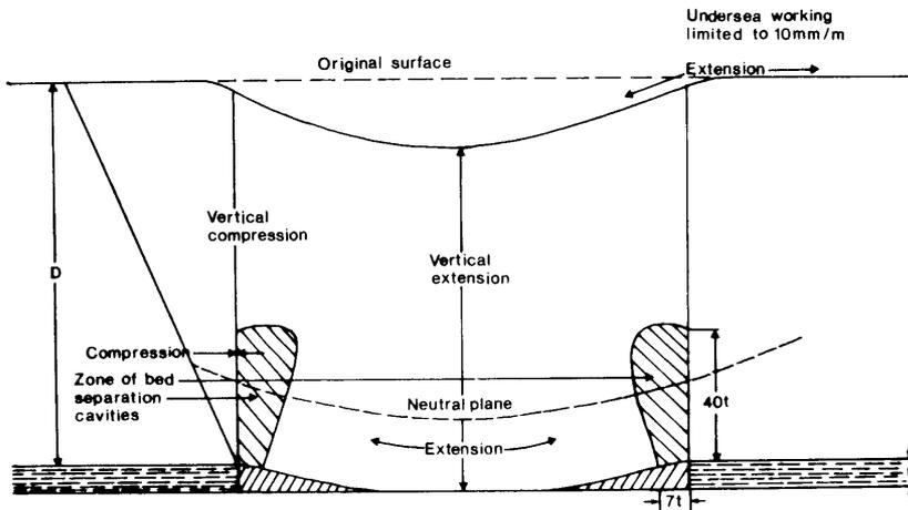
Fig. 2 Schematic Depiction of Stress Zones in Underground Mining
