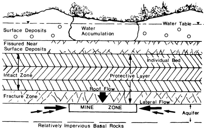
Fig. 6 Simplified scheme of Flow to a Mine through a Protective Layer
