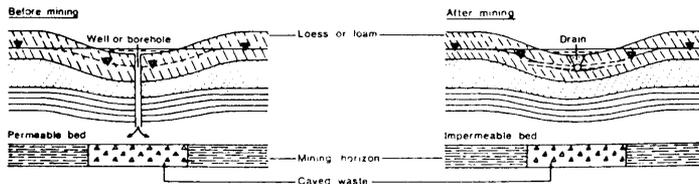
Remedial measure is to sink absorbing well or borehole into suitable receiving rock formation to drain surface water. The well drainage can also be assisted by mole or french drains.
