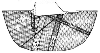
The best way for solution of such an underground flow problem is a numerical model with finite elements fitting the individual areas of different permeabilities.
