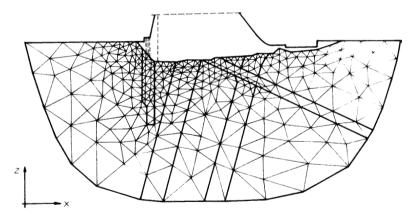
The results of the computer (we use for this the computer program POFEM (15 )) are then the distribution of piezometric head  $h\left(\mathbf{x},\mathbf{z}\right)$  drawn by a plotter
