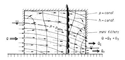
For using such a model concept it is necessary to estimate the dependence of  $K_{\rm V}$  and  $K_{\rm h}$  on the degree of saturation of the soil with water (14). The measurement of p or h is again possible by means of a vertical chain of mini-filters. As the computer code we are using the program VEREGO (13).
