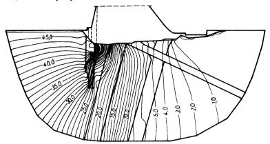
and the gradients of piezometric head  $\mbox{grad}\ h = f(x,z)$  also drawn by a plotter.
