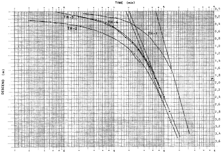
Figure 18. Hydrogram of descend - log. time, during TH-2 pumping test.
