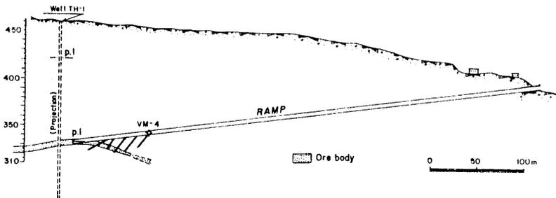
Figure 4. Access ramp showing artesian holes and TH-1 well.
