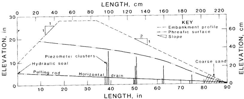
FIGURE 1. Cross section of laboratory embankment model.
