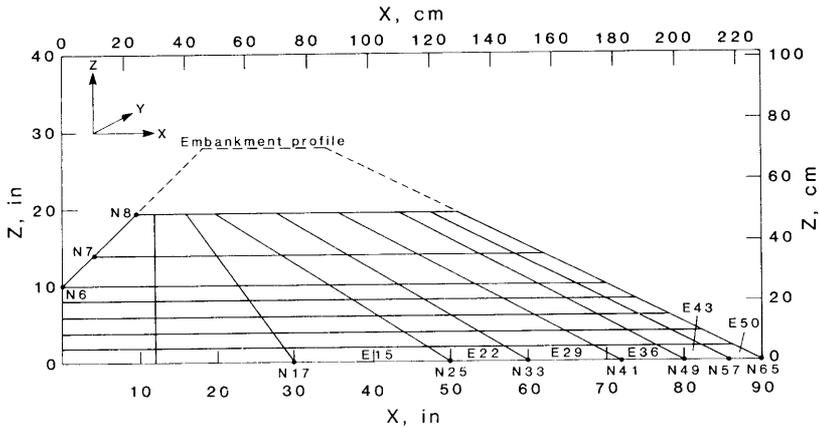
FIGURE 6. Cross section of three-dimensional mesh.
