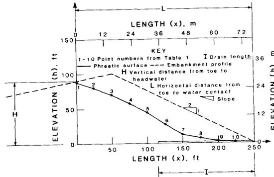
FIGURE 19. Embankment cross section plotted using dimensionless graphs.
