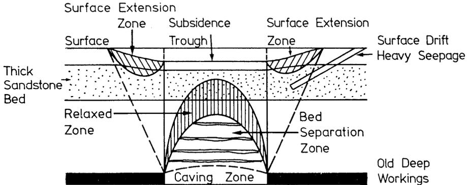
**Figure 11. Shallow Headings Passing Through Hard Strata Connected to Surface Extension Zone.**
