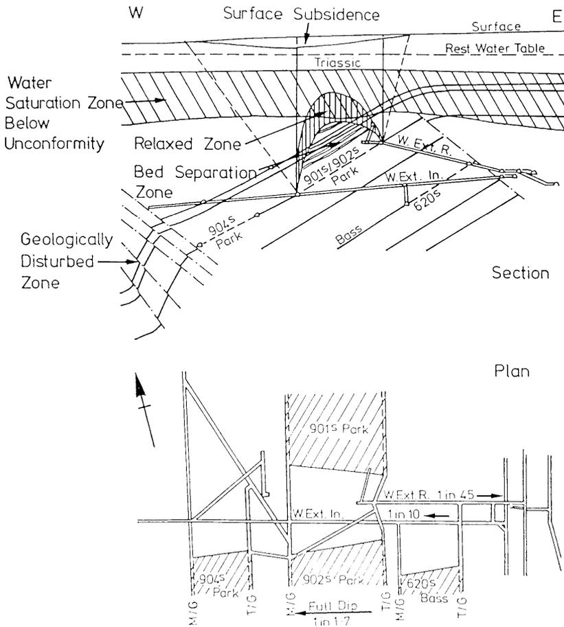
Figure 7. Water Problem of Steep Longwall Face Working Under a Saturation Zone Below Triassic.
