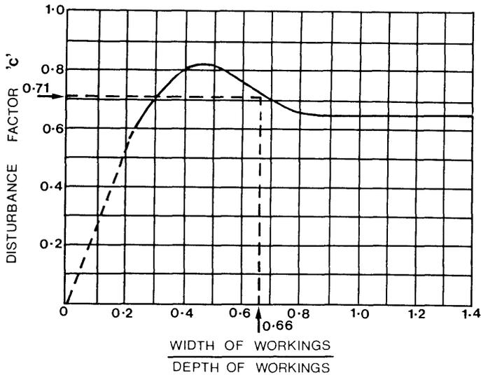
Figure 3 (a) - Disturbance factor for various ratios of width of working and depth, (Watson 1980)
