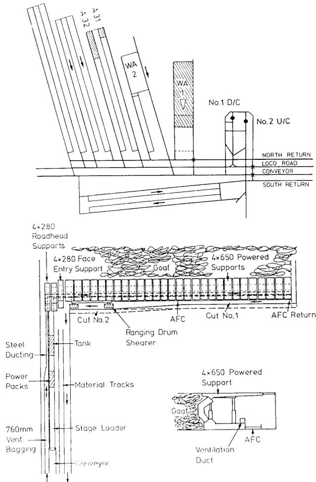
Figure 9. Layout of a Single Entry Face for Working Under a Major Aquifer.
