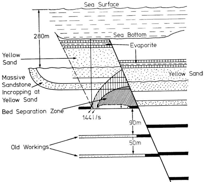
Figure 12. Under Sea Workings in Hard Stara in Faulted Zone.
