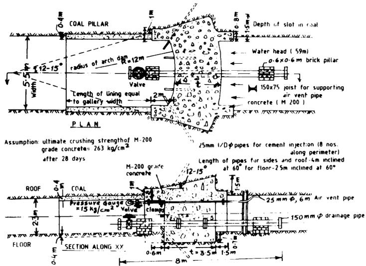
FIG. 3. CONSTRUCTIONAL DETAILS OF AN UNDERGROUND WATER DAM
