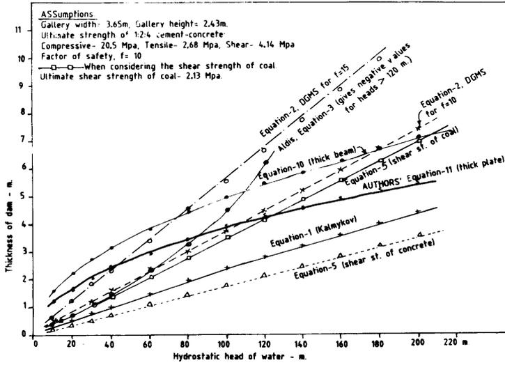
FIG-1. THICKNESS OF DAM AGAINST HYDROSTATIC HEAD- COMPARISION OF VARIOUS APPROACHES.
