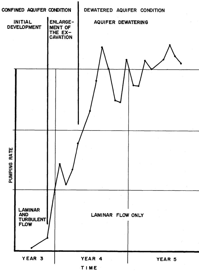
**FIG 3** MINE DEWATERING PHASES IN TYPICAL GOLD MINE
