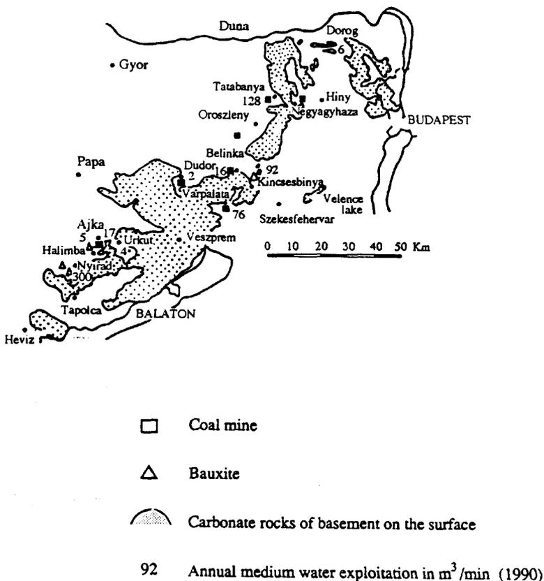
Figure 1 Mines in the Transdanubian range being endangered by water intrusions.
