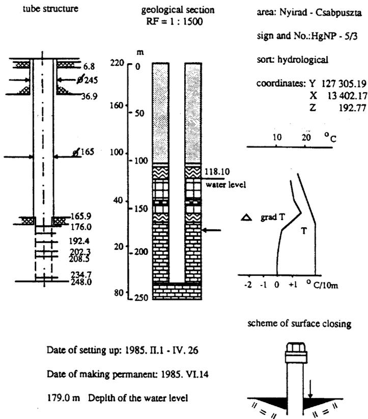
Fig. 6. One of the monitoring wells involved in the geothermal logging.
