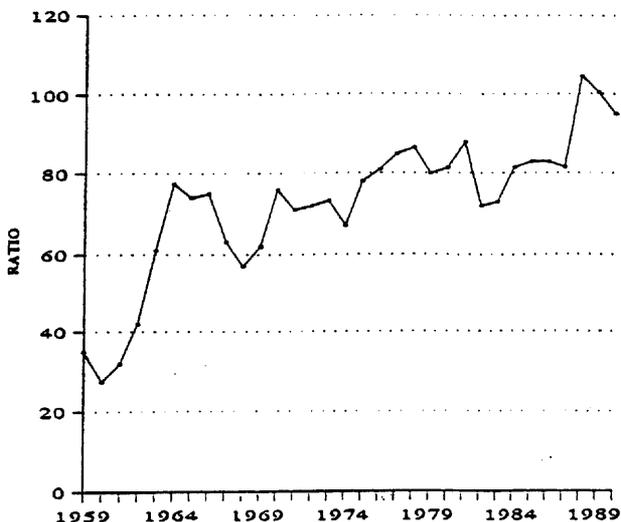
Figure 4. Ratio of volume of water pumped form the mine to tonnes of ore hoisted Konkola Mine (Mulenga 1991).
