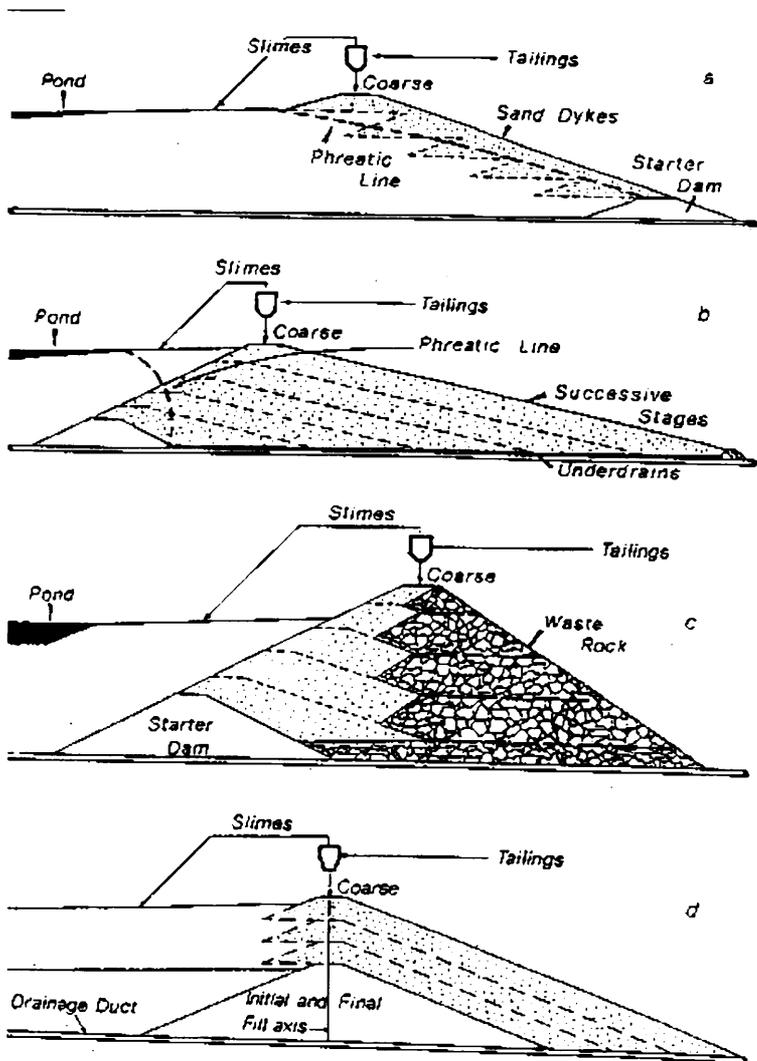
Figure 1. Basic methods of tailings dam construction: a, upstream method; b, downstream method; c, downstream method with mine waste rock; d, centerline method.
