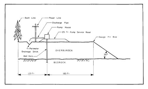
Figure No. 6 Section of Typical Pit Rim Arrangement
