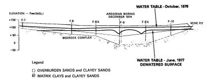
Figure No. 9 Reduction of Watertable a 14 acre area, overburden after prestripping averaged 28 feet and matrix averaged 20 feet. In this specific area, matrix yardage recovered was 300,000 cubic yards at a 71 percent recovery.
