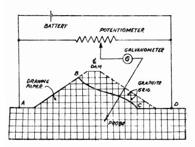
FIG. 1(b). Components of the Electrical Graphite Model
