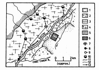
Fig.1 Hydrogeological sketch map of Bogovina coal basin. 1-Oligocene coal-bearing sediments, 2-tuffaceous rocks and andesite of Cretaceous age, 3-Cretaceous sandstone, 4-Mesozoik carbonates, 5-Paleozoik shales, 6-mine area, 7-cave with sinking water, 8-constant karstic spring, 9-intermitent spring, 10ponor, 11-perennial stream, 12-intermitent stream, 13-proved and assumed underground connection.
