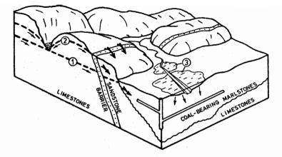
Fig.2 Schematic block-diagram of the Bogovina mine flood. 1-karst ground water level before the flood, 2-karst ground water level during the flood, 3-lakes formed by the Bogovina inundation.
