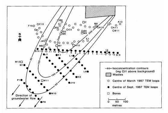
Figure 3. Model prediction of 50, 100 and 200 mg/l (above background) Cl contours at the water table after 6 years for  $\alpha_x = 30$  m,  $\alpha_y = 3$  m,  $\alpha_z = 0.3$  m and v= 100 m/y.
