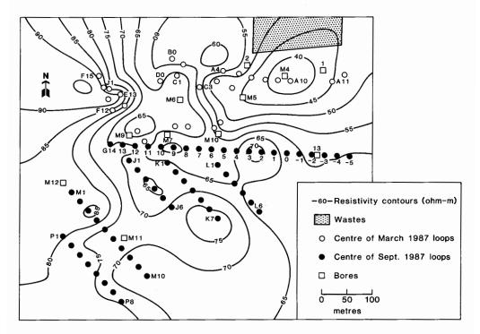
Figure 1. Resistivity contours obtained from computer inversion of TEM soundings at 5 ohm metre intervals, with borehole placements and centres of TEM loops marked.
