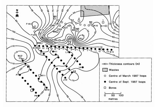
Figure 2. Thickness contours for the sand formation obtained from computer inversion of TEM soundings.
