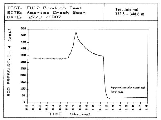
Fig. 6(a). Data from rod-string pressure transducer- Hole EH12, American Creek Seam
