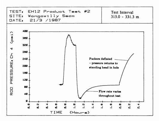
Fig. 5(a). Data from rod-string pressure transducer- Hole EH12, Wongawilli Seam
