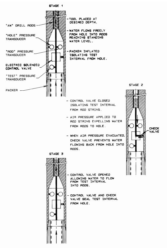
Fig.2. Principle of operation for production test
