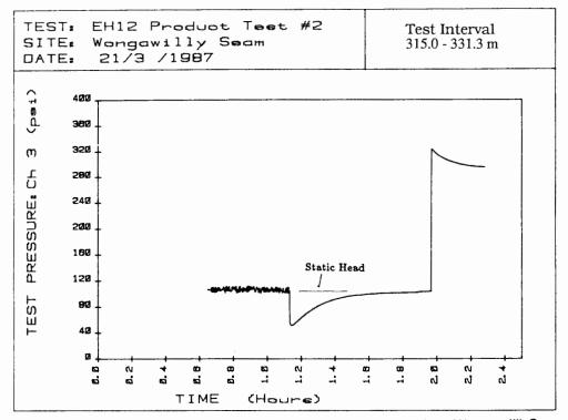
Fig. 5(b). Data from test interval pressure transducer- Hole EH12, Wongawilli Seam The Third International Mine Water Congress, Melbourne Australia, October 1988
