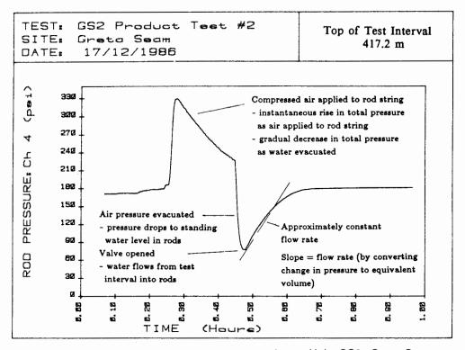
Fig. 4(a). Data from rod-string pressure transducer- Hole GS2, Greta Seam
