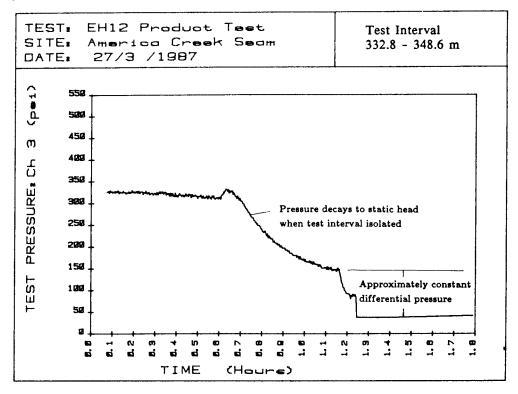
Fig. 6(b) Data from test interval pressure transducer- Hole EH12, American Creek Seam The Third International Mine Water Congress, Melbourne Australia, October 1988
