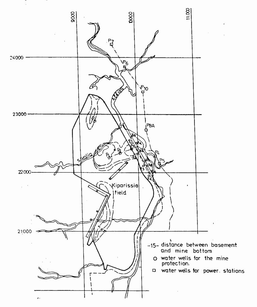
Figure 4: Kiparissia lignite field. Map showing the locations of water wells and isopaches of the sediments between basement and mine bottom.
