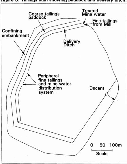
Figure 3. Tailings dam showing paddock and delivery ditch.
