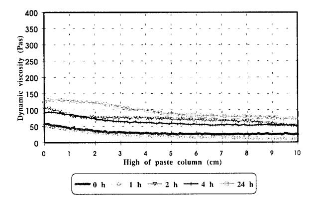
Figure 2.: Dynamic viscosity of paste as function of time (ball viscometer).
