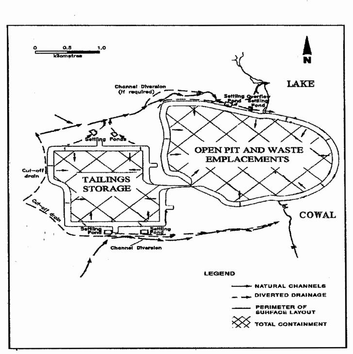
Figure 2: Mine site layout, drainage and water management plan (after NSR, 1996)
