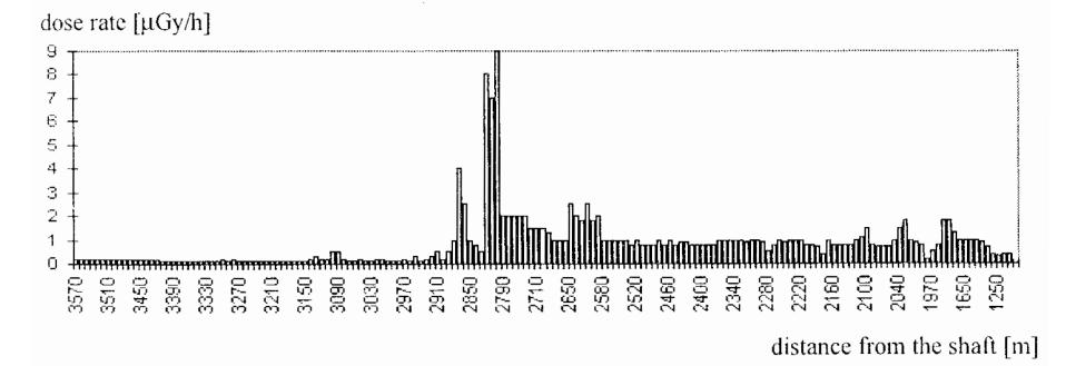
Fig.2. Gamma dose rates in a gallery with inflows of radium-bearing waters
