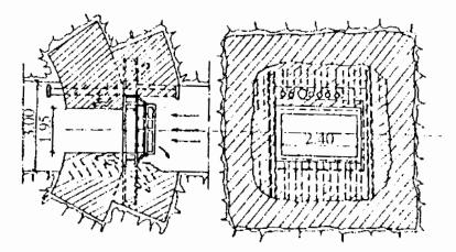
Fig. 4. Water gate diagram on the 13th horizon
