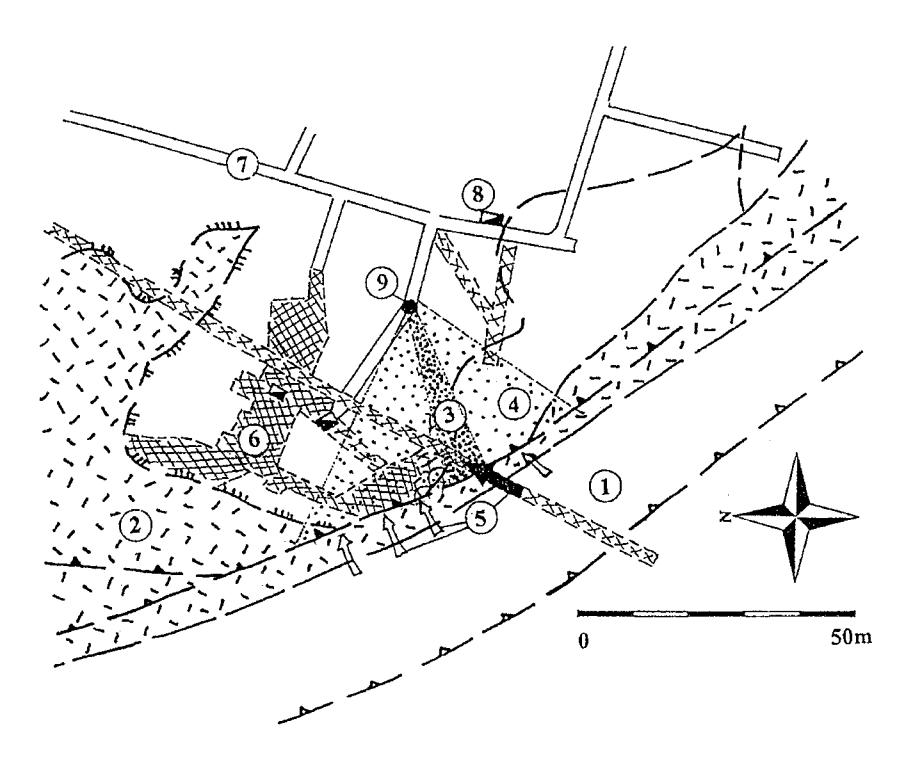
Legend: 1 - pervious layers with karst and fissured porosity, 2 - impervious layers, 3 - narrower injection area, 4 - broader injection area, 5 - foresen water inflows, 6 - backfllls, 7 - galleries, 8 - blind shafts, 9 - fan arrangement of injection boreholes
