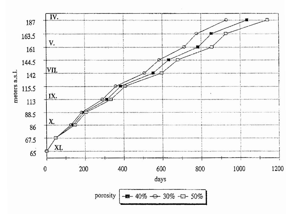
Figure 1: Forecast diagram of flooding the pit between the XIth and IVth levels
