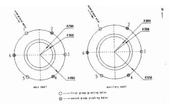
Figure 1. The locations of grouting holes
