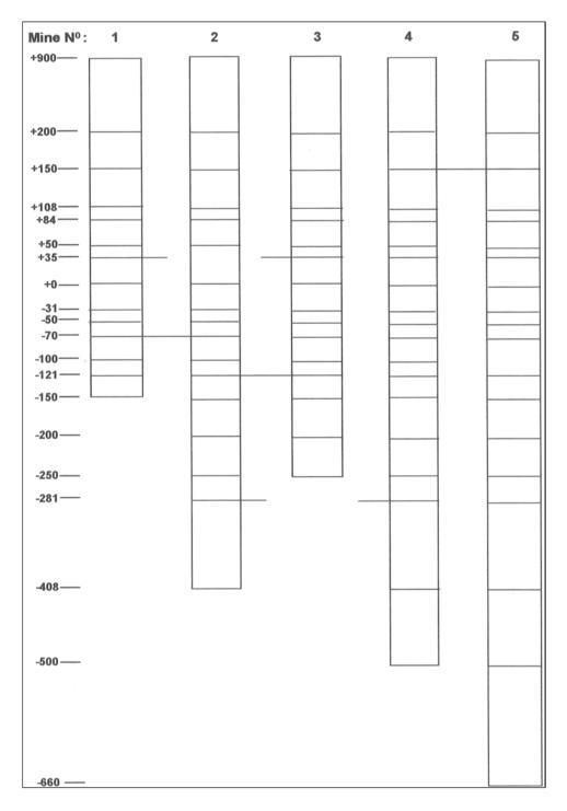
Figure 2 Scheme of connections between mines
