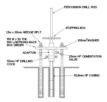
Figure 4 Percussion cover drill casing
