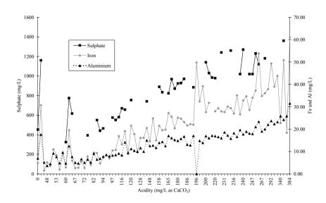
**Fig. 3.** Relationship between increasing acidity concentration and increases in concentration of Fe, Al and SO<sub>4</sub>, for tip leachate at Deerplay.
