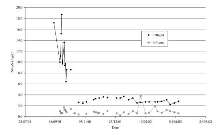
Fig. 4. Reductions in NH<sub>3</sub>-N concentration in effluent from the Deerplay RAPS over time.
