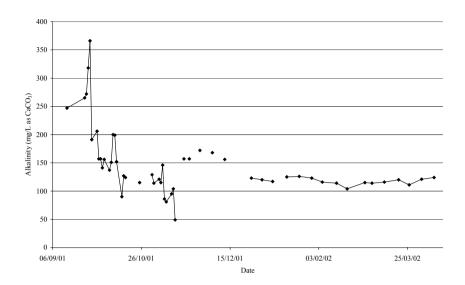
**Fig. 2.** Deerplay RAPS effluent alkalinity for the period September 2001 to April 2002 (Influent alkalinity is always zero)
