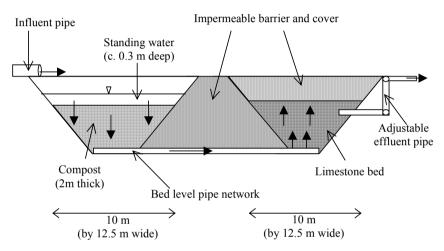
Fig. 1. Conceptual cross-section of the Deerplay RAPS (not to scale)
