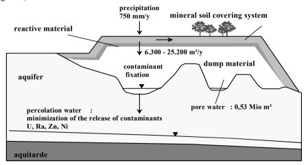
**Fig. 2.** Schematic cross section of a reactive covering system (Schneider et al 2002). The infiltration rate assumes the hydraulic breakdown of the soil cover.
