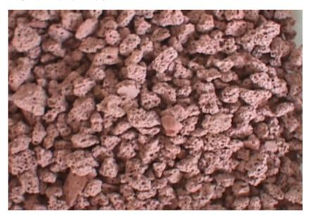
Figure 6. Granulated heavy spar bonded in foamed alumo-silicate (geopolymer)
