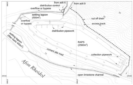
Fig, 5. Plan of passive treatment system
