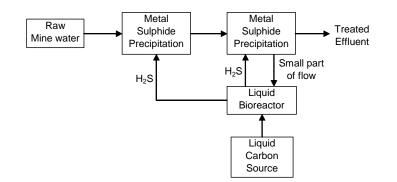
Fig. 4. Outline of a conceptual liquid bioreactor plant
