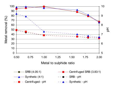
Fig. 5. A comparison of zinc precipitation and pH achieved by mixing of the metal solution with a synthetic sulphide/bicarbonate mixture and anaerobic digester overflow (T = 120min). The bicarbonate to sulphide ratios are shown in parentheses
