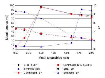
**Fig. 6.** A comparison of copper precipitation and pH achieved by mixing of the metal solution with a synthetic sulphide/bicarbonate mixture and anaerobic digester overflow (T = 120min). The bicarbonate to sulphide ratios are shown in parentheses
