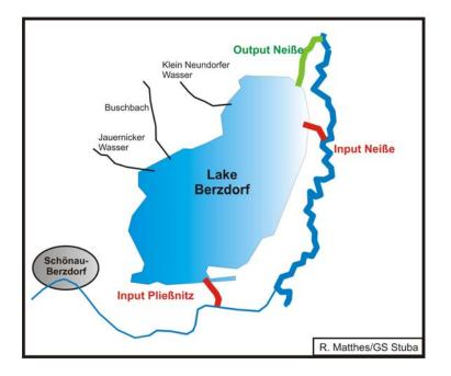
Fig. 1 Flooding system for the 'Berzdorf' pit
