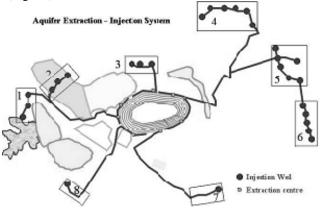
Fig 36. Drainage and injection wells for aquifer protection in the Las Cruces Project.
