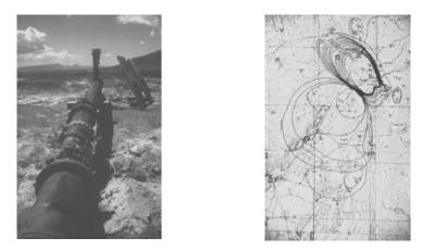
Fig 16. Re-injection well and conoids of the water table due to mine drainage and recharge.
