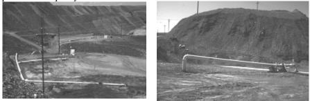
Fig 15. Wells for drainage from within and at Betze-Post mine's periphery.
