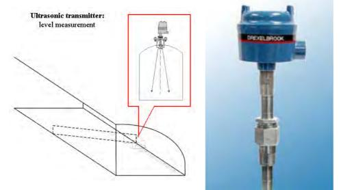
Figure 14: Flow measurement principle. Ultrasonic transmitter.
