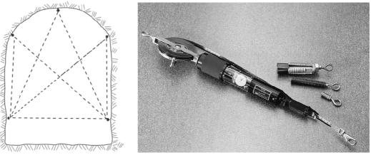
Figure 12: Tape extensometer
