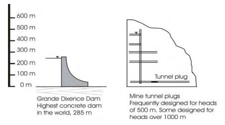
Figure 1: Comparison of Highest Dam to high Head Plugs [1]
