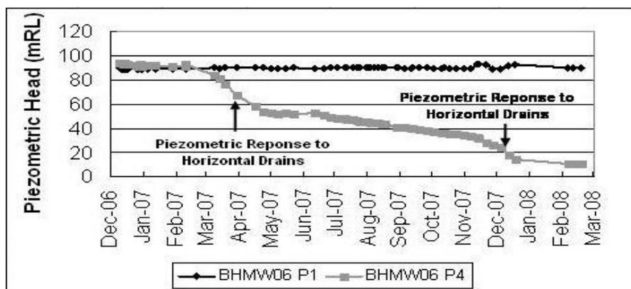
**Figure 15** Data from Vibrating Wire Piezometer BHMW07 at Batu Hijau showing no response to horizontal drains
