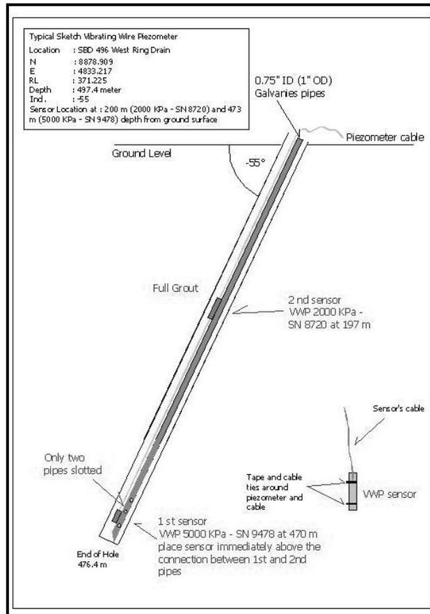
*Figure 12 Installation of a Vibrating Wire Piezometer at Batu Hijau in a horizontal drain*
