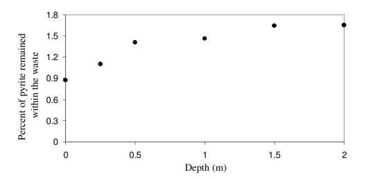
As the figure illustrates well, the rate of pyrite oxidation decreased sharply with depth up to 0.5 m, where oxygen concentration decreased rapidly. The process decreased gradually in the zone between 0.5 m and 1.5 m. For deeper layers (below 1.5 m) where no oxygen is available to oxidise pyrite, the pyrite oxidation reaction was completely ceased.
