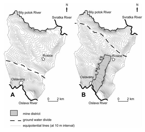
Figure 3 Original (A) and post mining (B) ground water flow conditions
