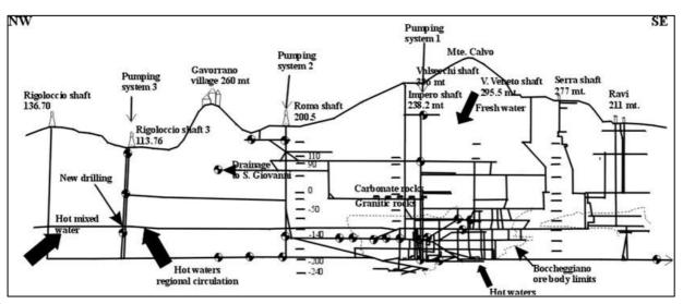
Figure 4 Scheme of main drifts and shafts in a vertical section across Gavorrano mine.
