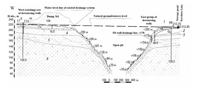
**Figure 2** Hydro-geological section along line 1 — 1 (see Figure 1): 1 — embankment; 2 — alluvial sediments; 3 — disintegration zone; 4 — interconnected strong fissuring zone; 5 — interconnected weak fissuring zone; 6 — uninterconnected weak fissuring zone.
