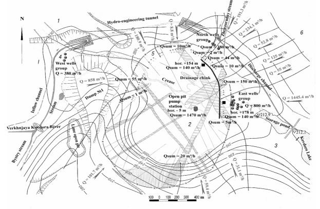
*Figure 1* Hydrodynamic structure of inflow groundwater forming in the open pit on 2000: 1 — alluvial sediments zone; 2 — broken disturbances zone; 3 — hydroisohyps; 4 — dewatering well; 5 — pit wall groundwater outlet; 6 — water current lines.
