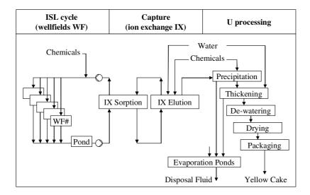
Figure 1 Schematic of ISL cycle, capture and uranium processing
