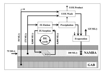
Figure 3 Schematic of water balance at Beverley with reference flow rates
