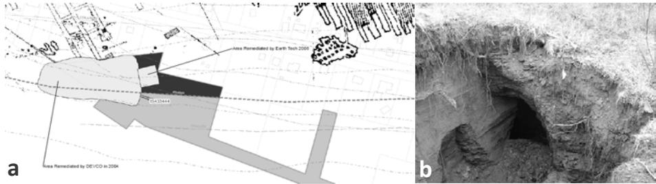
*Figure 3 Dominion No.3 Site – mining hazards: a) hazard map; b) hidden shallow workings*
