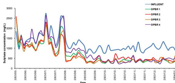
*Figure 1 Sulphate concentrations achieved for the DPBR columns relative to the influent sulphate concentration*
