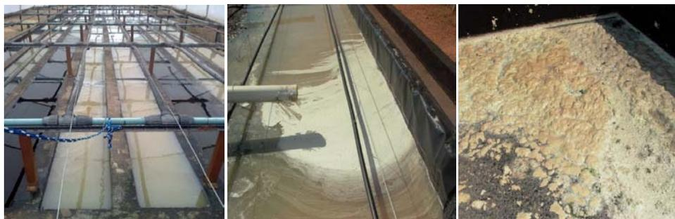
*Figure 3 Elemental sulphur formation in a. the BSOR, b. the DPBR and c. the splitterbox*
