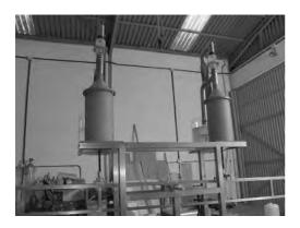
Figure 3 Photograph of the pumping system.
