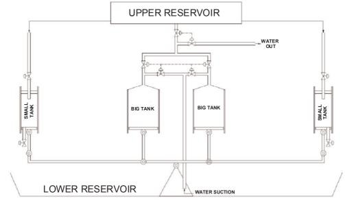
*Figure 4 Simplified schematic of the pumping system.*
