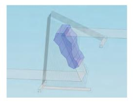
*Figure 4* Current freeze wall at McArthur River showing a cathedral ceiling "box" around ore zones.
