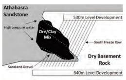
*Figure 3* Cross-section of ore and original freeze wall concept at McArthur River Mine.
