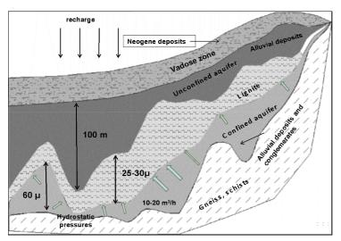
*Figure 4* Schematic section of Domeniko area.
