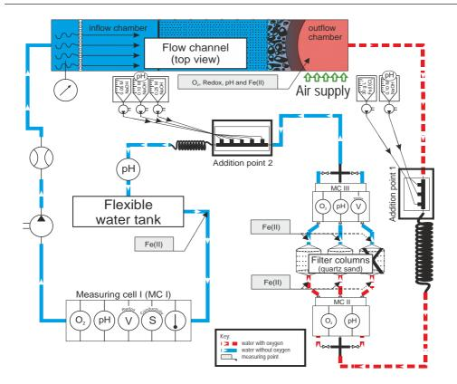
Figure 1 Experimental setup with illustration of the flow direction and the zones of  $O_2$ -bearing and  $O_2$ -free water. During the test period each of the filter columns can be exchanged by a third one. A 150 L flexible water tank is used as a storage reservoir for volume fluctuations and for buffering the effects of addition point 2.
