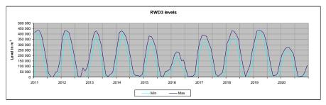
Figure 2 Simulated levels of the Tailings Return WaterDam 3
