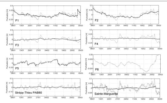
*Fig. 2* Example set of piezometric data (from January 6 to March 5, 2010). Raw data (dashed gray line) and data filtered for variations in atmospheric pressure and terrestrial attraction (black line).
