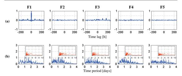
*Fig. 3* (a) Autocorrelation and cross-correlations of fluctuation rates of F1, with F1, F2, F3, F4 and F5. Data collected between November 28, 2009 and May 11, 2010. (b) Power spectral and cross-spectral densities of F1, with F1, F2, F3, F4 and F5. Densities are normalized. Densities are plotted as a function of the time period [days] (in blue) and as a function of frequency [cycle/day] (in red).
