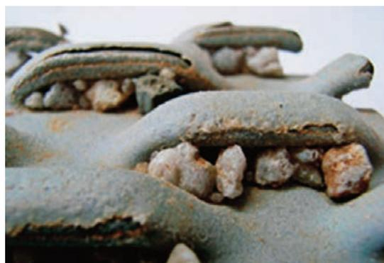
**Fig. 1** Clogged well screen with gravel debris after development pumping
