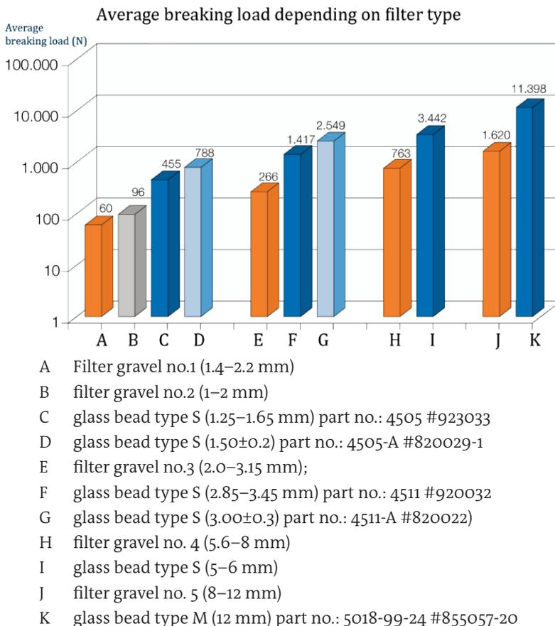
**Fig. 3** Magnitudes of breaking loads for filter gravel and glass beads at different granulations and bead sizes and mixtures at static load handling (TRESKATIS et al. 2010)
