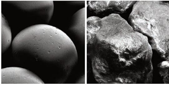
**Fig. 2** REM image of a glass bead compared to a filter gravel grain of the same grain size. The "smooth" surface of the glass bead prevents the formation of tensile stress when load is applied and reduces the agglomeration of incrustations (Treskatis et al. 2010).
