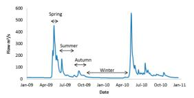
*Fig. 2* Typical annual flow hydrograph for the site (gauge number 65761 from OIVA database)
