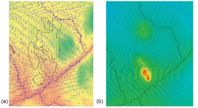
**Fig. 4** Groundwater contours at the mine site under (a) baseline and (b) life of mine conditions
