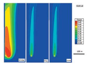
Fig. 6 Plume prediction model for life of mine (Year 18)
