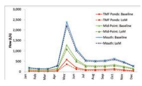
**Fig. 5** Baseline and life of mine (LoM) flow in the Niesajoki River, downstream of the TMF
